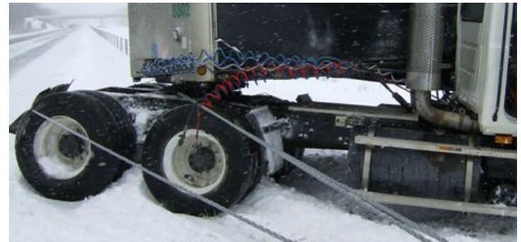
**CUT THE CABLES ONLY AS A LAST RESORT.** Cutting cables should only be considered under life or death situations where time is absolutely critical, and other alternatives for loosening cables are not feasible. Cutting cables will require a cable splice or a complete cable section replacement, which is time consuming and costly.
